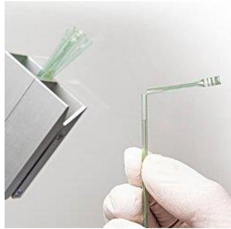
The cutting procedure is shown in the picture above. First, pull the straw down through the gap in the SG Cutter. It is important to hold the straw close to the cutter to protect the capillary inside. Bend the cut-off part on the top of the straw.
