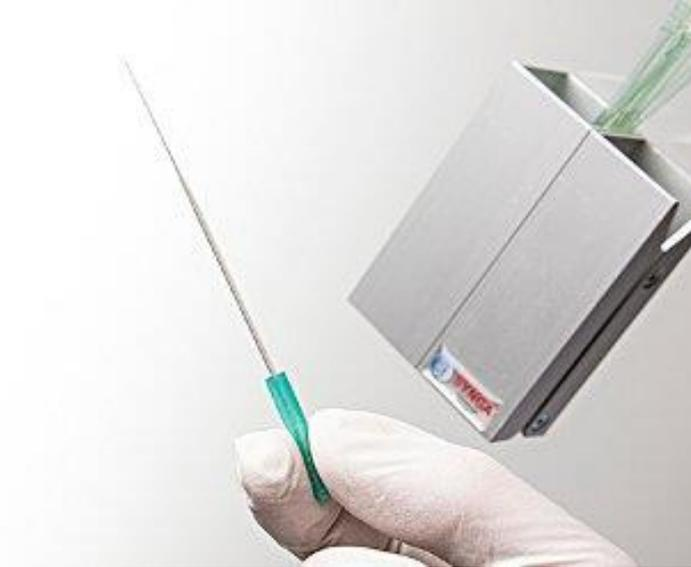
Pipette is now ready for use, with a penholder or without it. Notice the right cutter mounted on the right wall.
