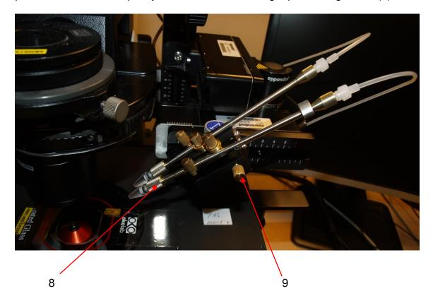
Finaly you can adjust the forth and back position of the front capillary holder (8) with the forward adjustment wheel (10).
